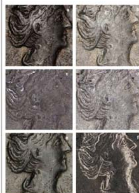
Fig. 2. Coin A, obverse (detail). a) RTI capture UCL dome; b) RTI capture Cyl dome; c) RTI capture RBINS Minidome, albedo mode; d) RTI capture RBINS Minidome, ambient mode; e) RTI capture Southampton dome; f) Focus stacked picture.
