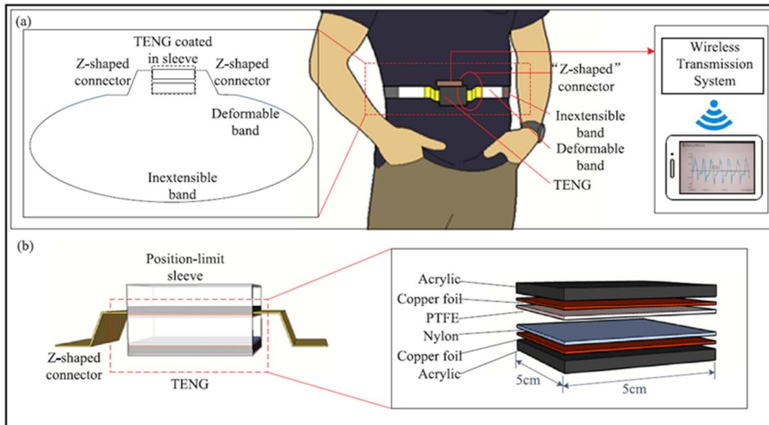
Fig. 1. Waist-wearable respiration sensor and wireless transmission chip. (a) Schematic design of the respiration sensor with a wireless transmission chip, (b) schematic structure of the contact mode TENG.
