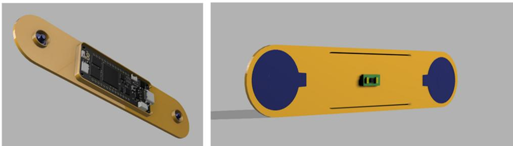
Figure 2.2. On top of the patch (left image) is a microprocessor unit with opto-acoustic signalization. On the underside (right image) there is one pair of ECG sensing electrodes with a PPG sensor placed between them.
