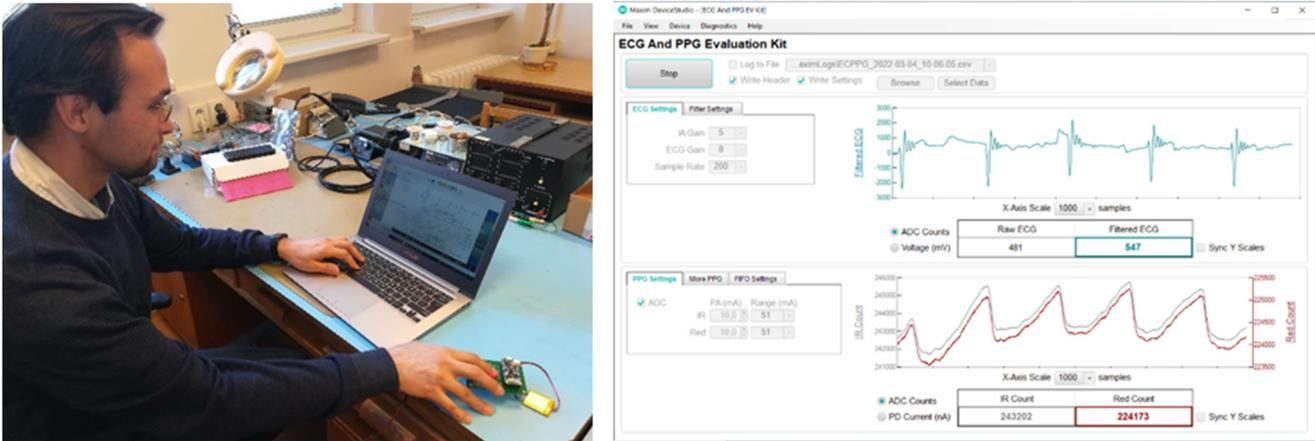
Figure 2.1: The image on the left shows the control program from Maxim integrated sensor with the measured PPG and ECG signal waveforms.
