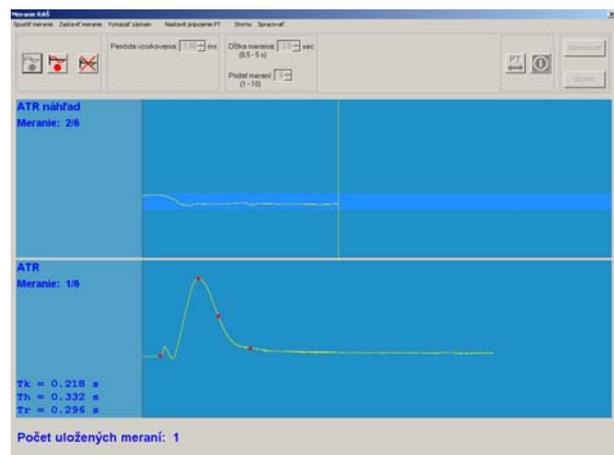
Figure 11: Screenshots of the evaluation of the ATR signal with marked time instants TK, TH and TR.
