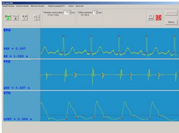
Figure 12: Screenshot of the evaluation of cardiovascular signals. Automatically detected time instants Q and R in the ECG signal, S2 in the PCG signal, upstroke and incisure in the CAR signal are marked in the recordings and used for computation of systolic time intervals.
