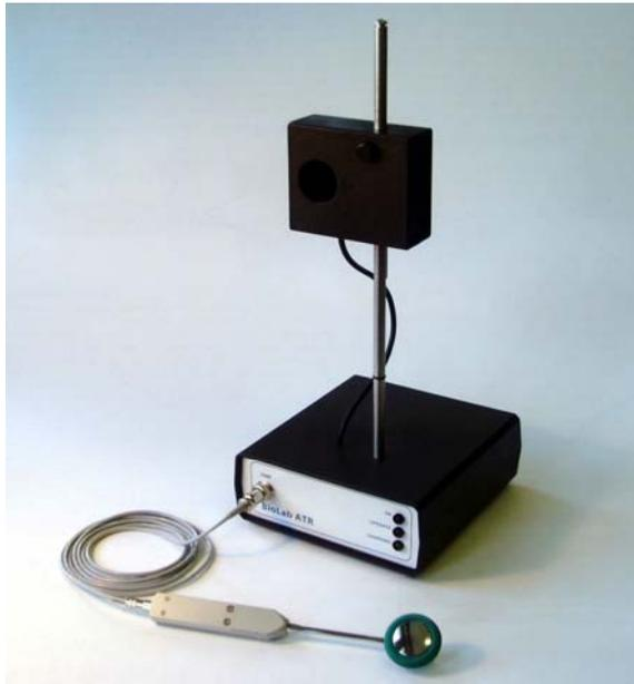
Figure 5: BioLab ATR smart sensor module with optoelectronic sole movement sensor and synchronized stimulating neurologic hammer.
