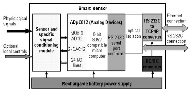
Figure 4: Simplified block scheme of the BioLab smart sensor module
