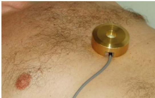
Figure 9: PCG measurement using the ADInstruments MLT 201 Cardio Microphone
