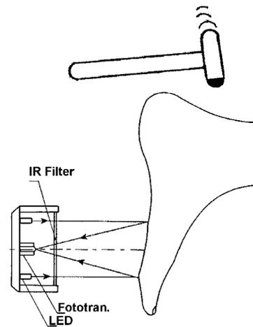
Figure 6: Principle of the ATR signal measurement.
